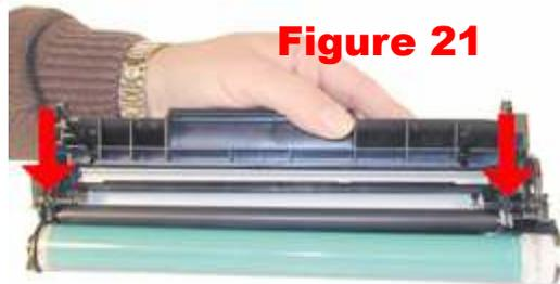
15. The waste bin section is complete. Set aside and bring the toner hopper section in front of you.
