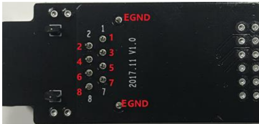
Figure 4. Eport-E20-PIN Pins Map
