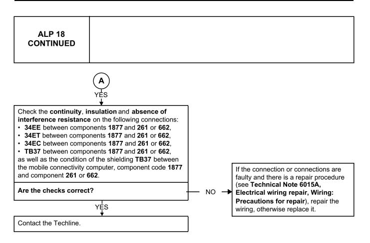
Carry out another fault finding check on the system. Deal with any faults.
