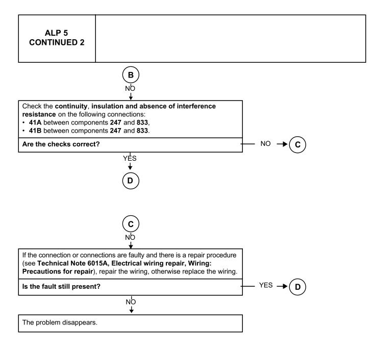
AFTER REPAIRDeal with any faults displayed by the diagnostic tool.<br/>Clear the computer memory.<br/>Carry out a road test followed by another check with the diagnostic tool.
