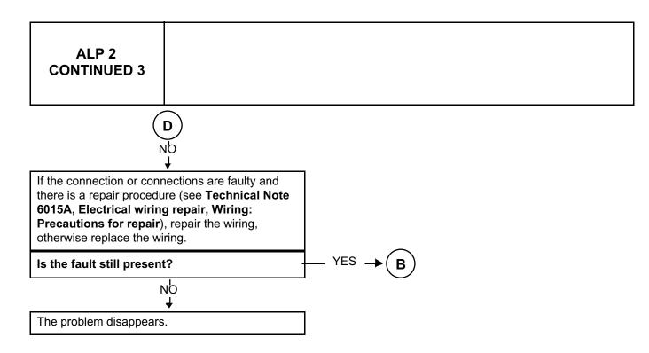
AFTER REPAIRDeal with any faults displayed by the diagnostic tool.Clear the computer memory.<br/>Carry out a road test followed by another check with the diagnostic tool.
