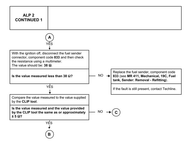
AFTER REPAIRDeal with any faults displayed by the diagnostic tool.Clear the computer memory.<br/>Carry out a road test followed by another check with the diagnostic tool.
