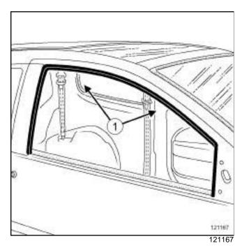
☐ Partially remove the upper section (1) of the front side door run channel.
