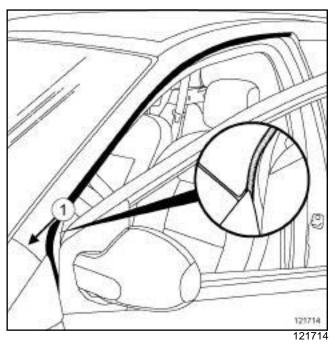
☐ Partially remove the lower section of the paper protecting the double seal cement bead (1).
