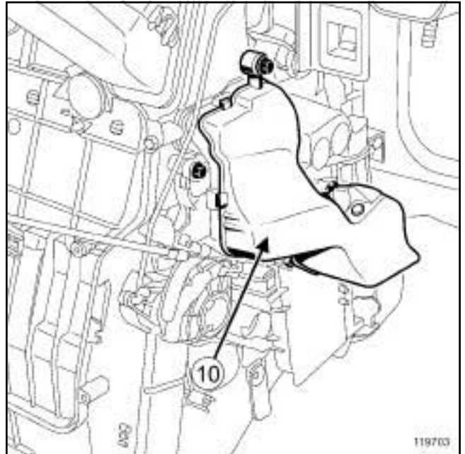
Front right-hand footwell air distribution duct (10)
