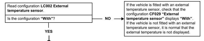
Check that **LC067 "External temperature display"** is **"WITH"**. Otherwise perform **CF171 "Temperature display"**.
